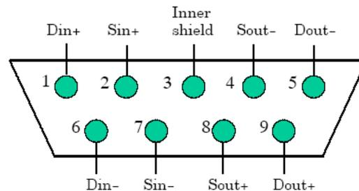
SpaceWire users have recognized these issues. NASA Goddard Space Flight Center has commissioned an alternative connector [4] that is rather larger than the micro-D but which presents much less of an imbalance or discontinuity to the signals. 4Links have described mitigation techniques for the EMC emissions that can be implemented with low-cost components and with negligible additional mass [5].
